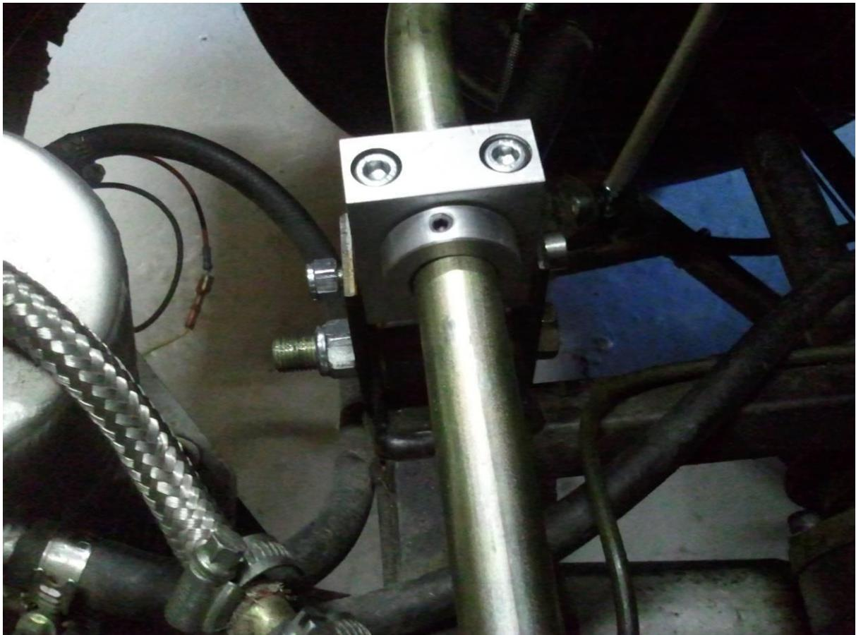
The bar is now secure and in the correct place, it should however be able to swivel up and down. If not then a small amount of copper slip or grease may be needed to allow the bar to do so.
