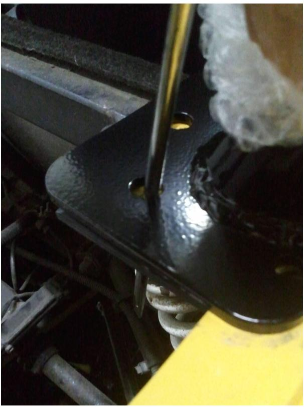
The Short 10mm bolts will go through the holes that size and the  $2 \times 8$ mm bolts will go through the holes their size. Below is what it should look like, with the one bolt upside down to the rest on the passenger side. Also taking care when fitting the rollbar that the seat belt eyelets don't catch the rollbar (particularly on the passenger side).
