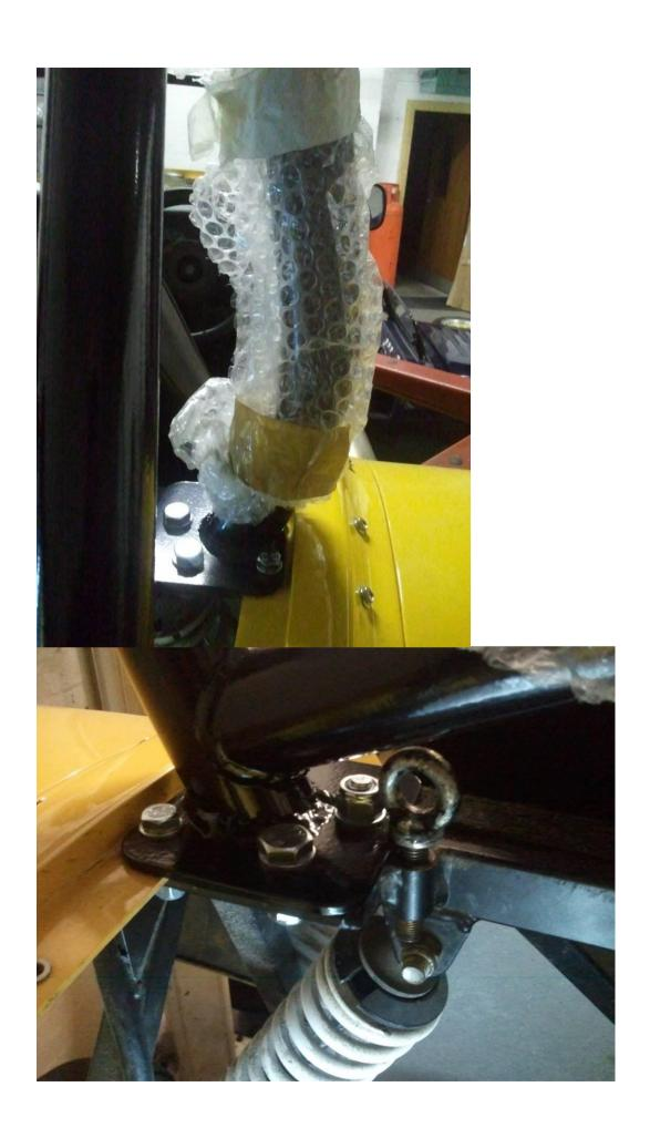
The Gold anodized parts need to be bolted into place on the U brackets that are welded to the chassis, using two of long 10mm bolts.
