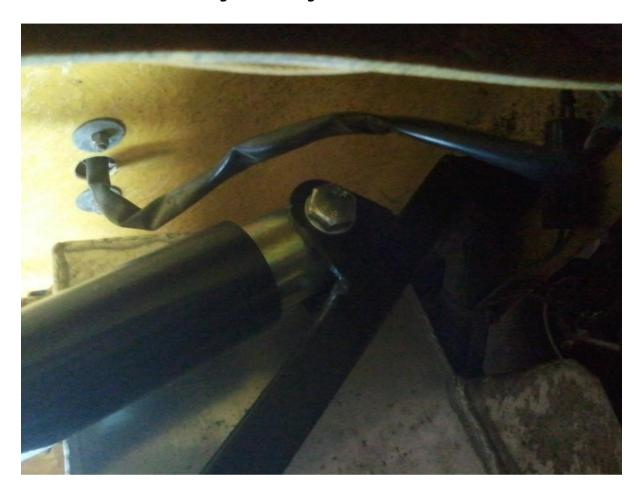
Finally the gold anodized tubes need to be bolted to the rollbar. To do this it is easiest to do it on the car. With the car in the air and the rear wheels off, if you pilot drill a hole going diagonally through the centre of bar so when it comes out of the other side it misses the fuel tank. This then needs to be drilled with a 10mm drill so the bolts will go through. If you prefer you can remove the rollbar to do this.
