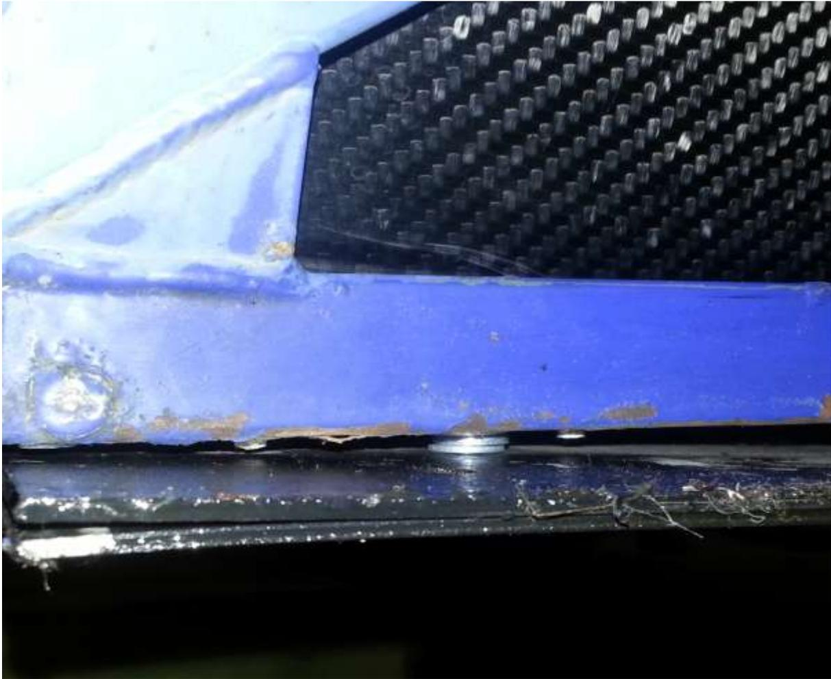
The front of diffuser can now slip onto this plastic and slide between the plastic and chassis. This keeps the front of the diffuser nice and secure. You can push the diffuser further forward, by cutting some slots where the bolts are so the diffuser can slide further forward.
