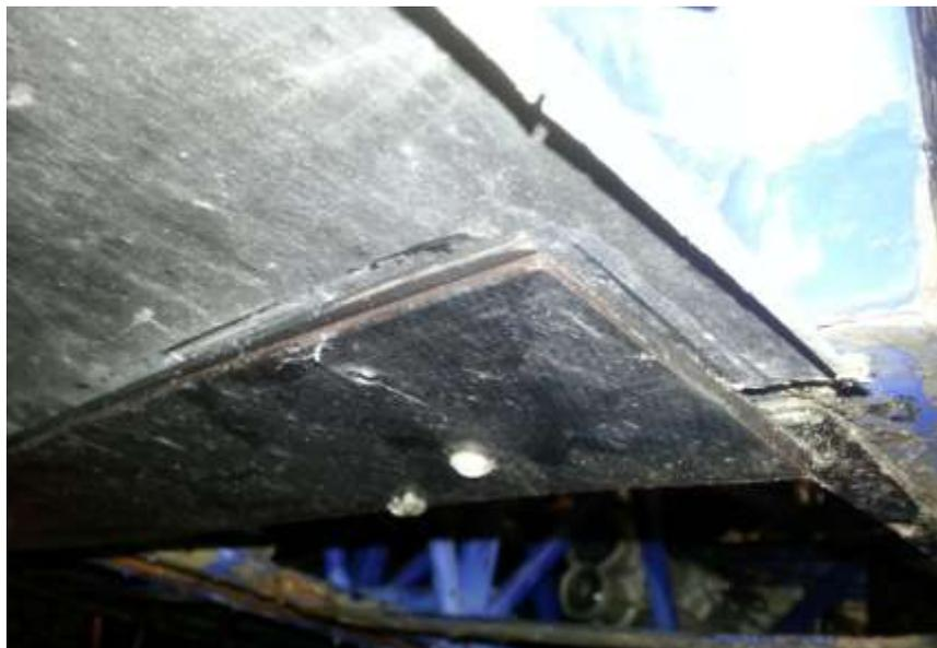
The rear of the diffuser can now be secured using either some bonnet pins or dzus fasteners.
